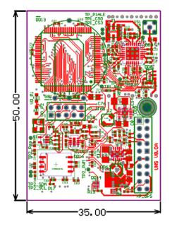
The digital receiver computes position, updates ten times a second, measures position to 5 meters, and measures velocity to 0.1 m/s.
